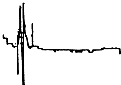
Fig. 3. Chromatogram from analysis of microemulsion without lysine clonixinate salt.
